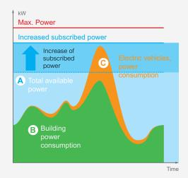
This solution consists of increasing the power subscribed to the energy supplier to maintain the same consumption model. It implies an increase in the cost of the subscription and the trigger threshold can be exceeded. Thus the continuity of service of the building could be impacted.
