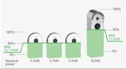
The energy will be delivered according to an equal percentage, in this example: 51%. Details
