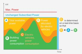
Setpoint "D" is adjusted in real time according to the consumption of the rest of loads in the building, to maximize the power allocated to charging electric vehicles.
