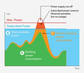
The installation of charging stations in an existing electrical installation can have a significant impact due to the power level required by electric vehicles to charge.
