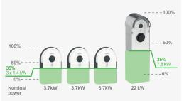
When reaching the minimum current setpoint of a charge point, its current level will be maintained so that the EV keeps charging.
